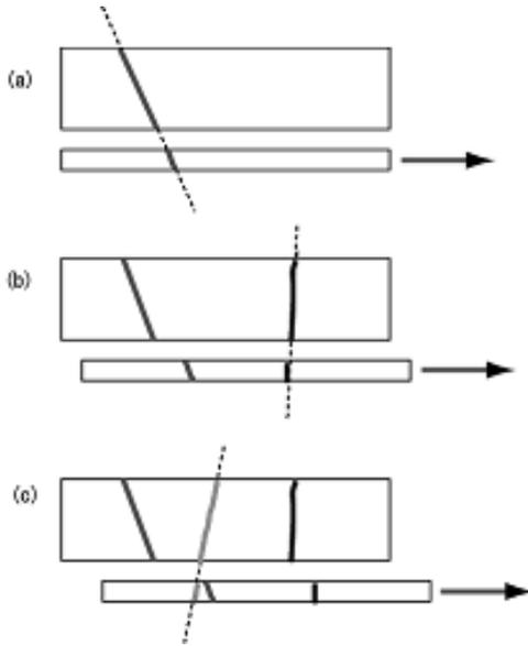
Fig. 3: The schematic view of emulsion shifter. In the upper panel (a), emulsion chamber and emulsion shifter are aligned each other, and then the shifter part are moved to the right direction like (b) and (c). The registered track positions between them show proper displacements.
