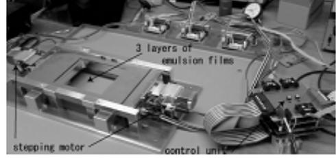
Fig. 8: 1/10 scaled flight model of multistage emulsion shifter.
