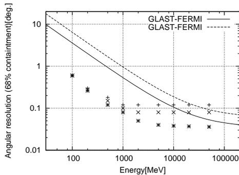
Fig. 1: Simulation results of angular resolution dependencies on gamma ray energies in a few cases of emulsion readout unit. Solid line and dashed one represent the angular resolution reported by GLAST team. Data symbols (plus, cross, asterisk) mean the emulsion digitizing readout accuracy of  $0.3\mu\text{m}$ ,  $0.2\mu\text{m}$  and  $0.1\mu\text{m}$ , respectively.
