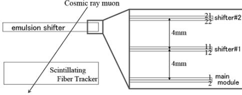
Fig. 5: Schematic views of experimental setting of multi-stage emulsion shifter applications. Emulsion shifter part consists of 6 emulsion films including 2 fixed layers. The scintillating fiber tracker provided the event time stamp for each atmospheric muons.
