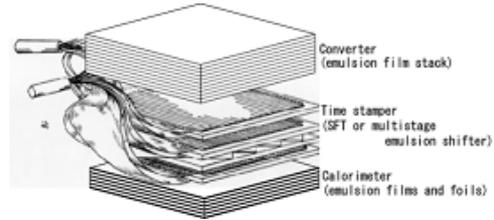
Fig. 2: The conceptual design of emulsion telescope. Though scintillating fiber tracker (SFT) systems would be used to get time stamp information of cosmic gamma ray events originally in this figure, it is going to be replaced by multistage emulsion shifter system, described in the following sections.
