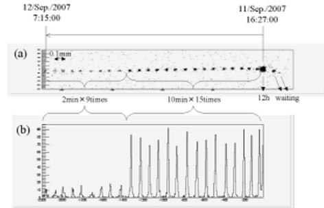
Fig. 4: (a) Observed track displacement at shifter part and (b) the track density at each displacement. The number of tracks at each displacement are proportional to the time duration.
