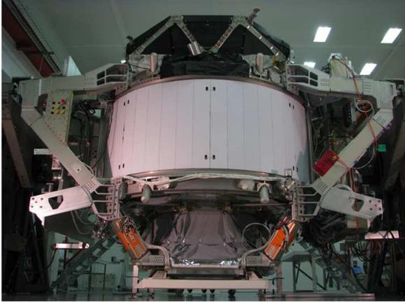
Fig. 6. The (pre) assembled AMS-02 detector.
