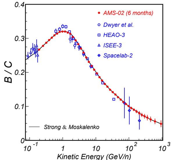
Fig. 3. Available measurements of the B/C flux ratio and the expected AMS-02 resolution, statistical errors only.
