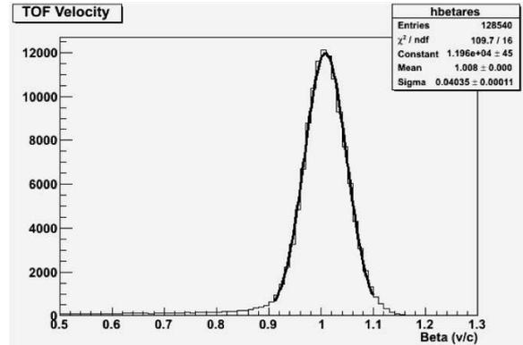
Fig. 7. The  $\beta$  measurement resolution of the TOF sub-detector.
