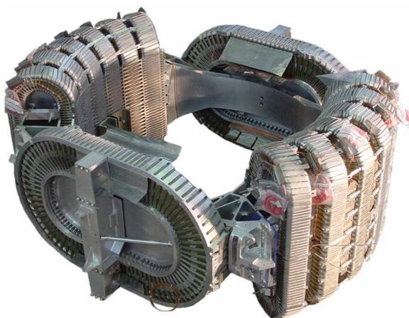
Fig. 1. The AMS-02 superconducting magnet.
