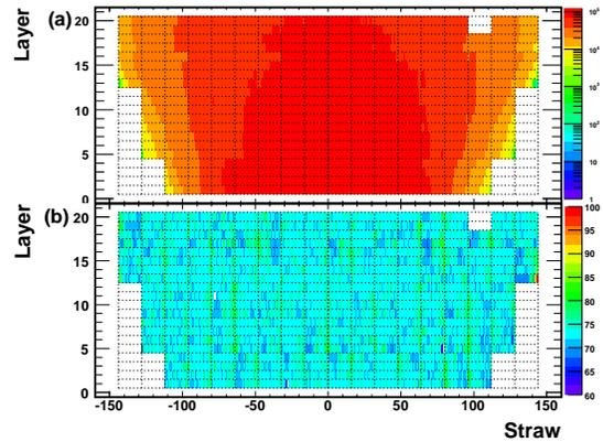
Fig. 7. Track occupancy (a) and gas gain homogeneity (b) with cosmic muons. The obtained average deposited energy is  $73.56 \pm 1.81$  ADC counts and overall signal inhomogeneity is 2.5% after corrections. The palette scales show the number of hit per straw tube (a) and the most probable value of the Landau fit on each straw tube (b). Two straw modules mounted 19th and 20th layers are excluded due to an unstable preamplifier chip which was replaced after preintegration stage.
