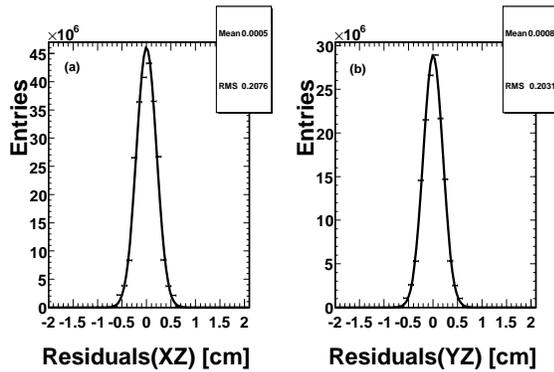
Fig. 5. Distribution of the residuals of the straw tubes from the reconstructed particle tracks in both xz (a) and yz (b) planes. Two residual plots are almost identical in the position resolution of 2.0 mm
