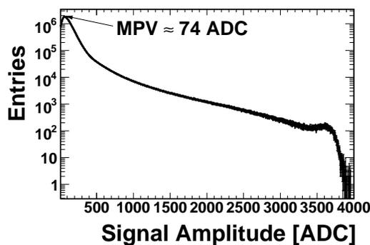
Fig. 4. Distribution of energy deposited on single straw tube by single muon track events. The ArCO<sub>2</sub> gas is supplied at a constant flow rate of 1 l/h and the same high voltage of 1400 V is applied after calibration of each UHV channel.
