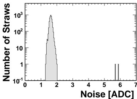
Fig. 6. The distribution of noise for all straw tubes. The average noise is  $1.62 \pm 0.08$  ADC and spread of the noise is within 5% except of two noisy channels out of 5248 channels.
