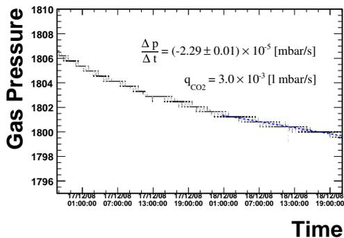
Fig. 3. Gas tightness testing for a TRD gas volume of 230 liter with ArCO<sub>2</sub> (80/20) at 1800 mbar and constant temperature of 23.0 °C. Pressure sensors monitor on both gas inlet(upper black dots) and outlet sides.
