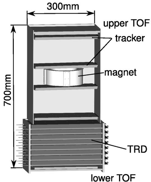
Fig. 3. A 3D model of the PERDaix detector.
