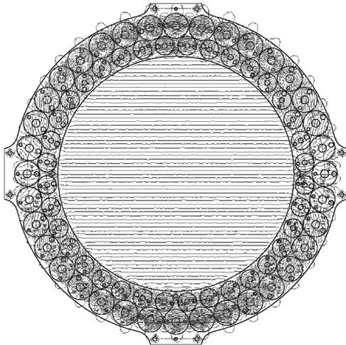
Fig. 4. A mechanical drawing of the PERDaix permanent magnet array with magnetic field lines calculated with the finite element method.
