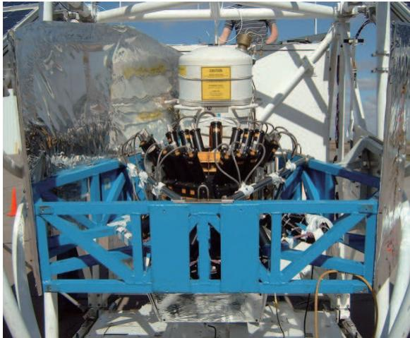
Fig. 2. The cryostat as it was situated in the balloon gondola. The view is from above and in front of the detectors. Note the white LN2 dewar behind the cryostat and the active BGO shielding surrounding the sides and bottom of the cryostat. For the LDBF, the size of the signal cables (visible here) will be greatly reduced. An active collimator will also be added around the cryostat, constraining the field of view further.
