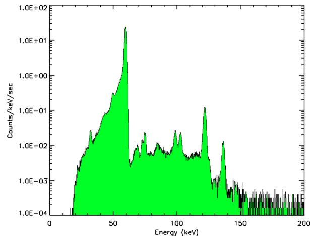
Fig. 3. Energy spectrum obtained during the end-to-end test of the electronics boards. Data shown are for single-site events (i.e., the event contains only two strips – one from each side of the detector). Clearly seen are the  $^{241}\text{Am}$  59.5 keV line and the  $^{57}\text{Co}$  lines at 122 keV and 136 keV. Other weaker lines are mostly from  $^{241}\text{Am}$ .
