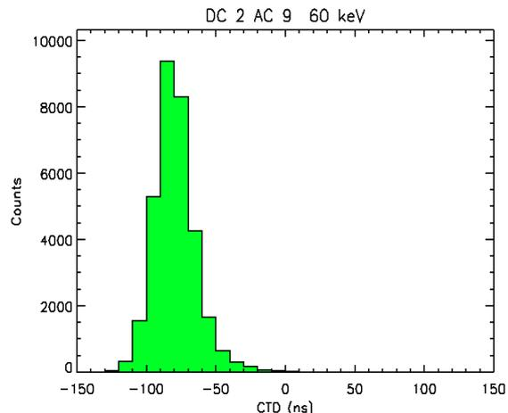
Fig. 4. More data from the test setup: CTD histogram of a single pixel (AC 9, DC 2), showing events that are energy-selected to be photoabsorptions of 59.5 keV photons. Since the CTD is a proxy for depth in the detector, we see the expected result that the 59.5 keV photons do not penetrate far into the detector (the incident detector surface is at approximately -100 ns, the far side is at approximately +100 ns).
