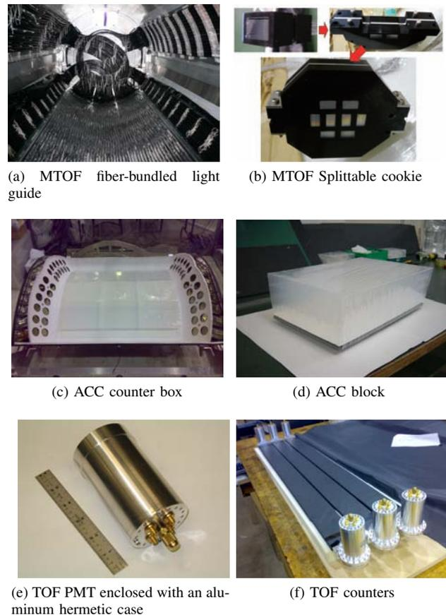
Fig. 3: Newly developed detectors for BESS-Polar II
