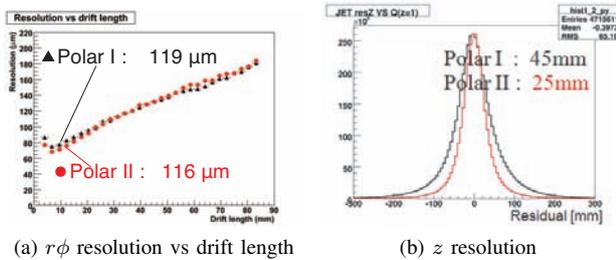
Fig. 8: (a)  $r\phi$  and (b)  $z$  resolution of the JET chamber in comparison with those from BESS-Polar I.
