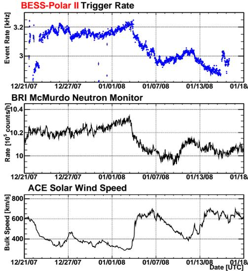
Fig. 7: Top: BESS-Polar II trigger rate, Middle: neutron monitor, Bottom: solar window speed
