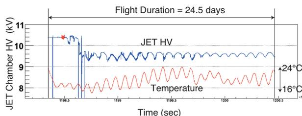
Fig. 6: Fluctuation of JET chamber High voltage, together with JET chamber gas temperature.
