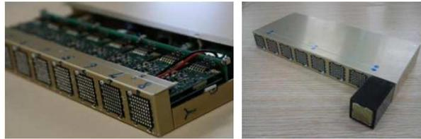
Fig. 2. Left picture shows a FEC unit developed to read out MAPMT. One MAPMT is attached to the FEC in the right picture. The FEC unit contains 16 chips of VA32HDR14 to read out 8 MAPMTs. Analog signals of 512 channels from MAPMT are processed and digitized by 16 bits ADC.
